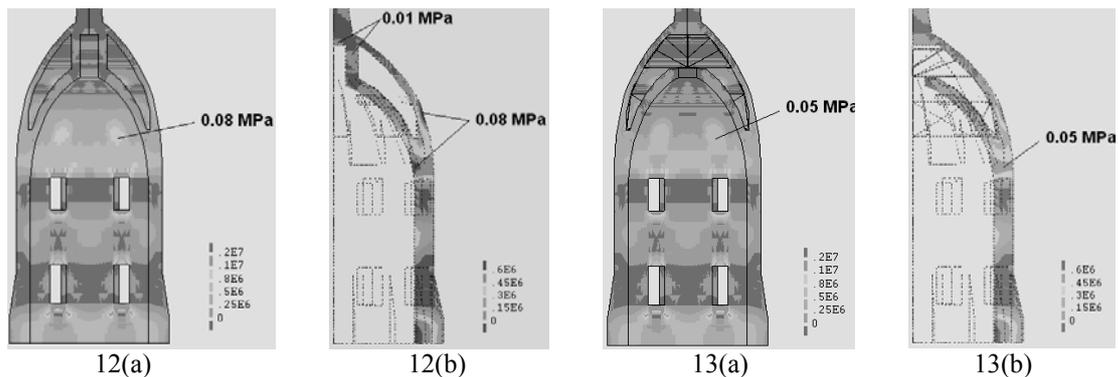
Figures 12(a,b) : Phase 2 - Tensile Stress Map over the walls (a) and across the thickness of the wall (b).
