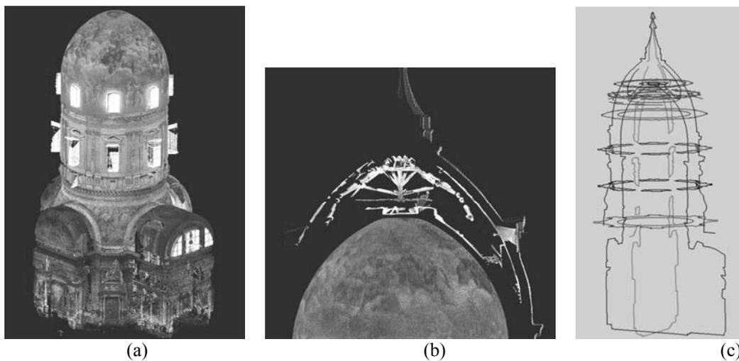
Figures 9(a,b,c) : Scanner digital images of the dome and plan and sections in Cad environment.
