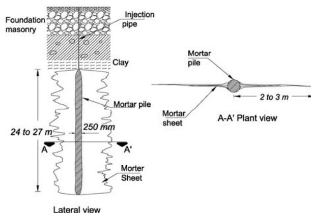
Figure 4 : Mortar inclusions for reducing soil compressibility (adapted from Santoyo et al., 2005)
