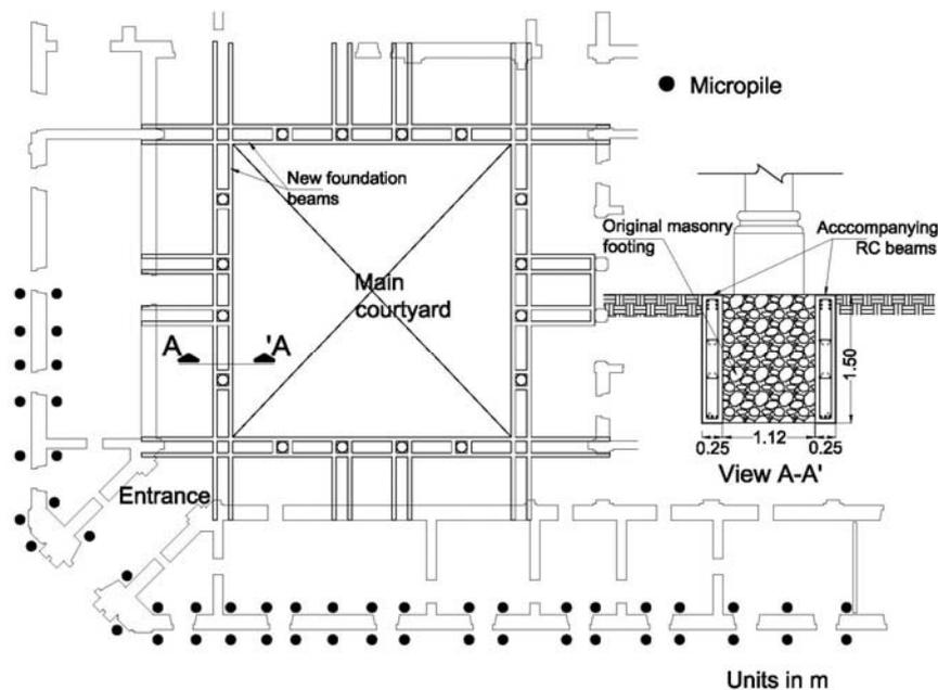
Figure 7 : Foundation strengthening with micropiles and accompanying RC beams
