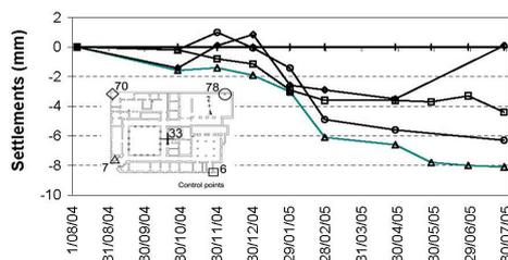
Figure 9 : Evolution of differential settlements during and immediately after installing micropiles
