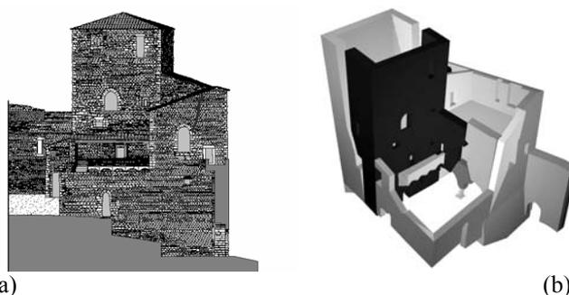
Figure 3 : (a) Cracking on WallA2; (b) Reconstruction of general displacements
