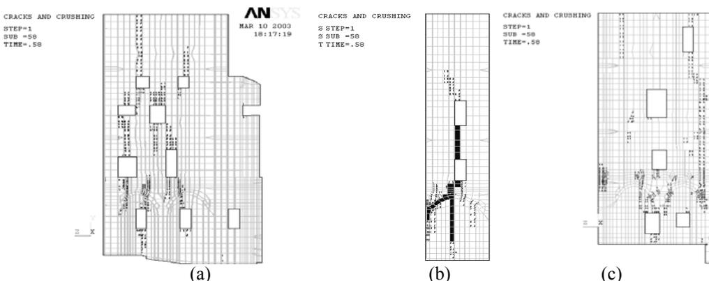
Figure 7 : (a) Cracking path on Wall T2; (b) Cracking path on Wall T4; (c) Cracking path on Wall T1
