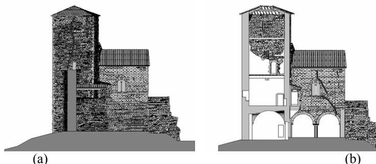
Figure 2 : (a) Cracking on Great Tower (Wall T4) : (b) Cracking on WallA3
