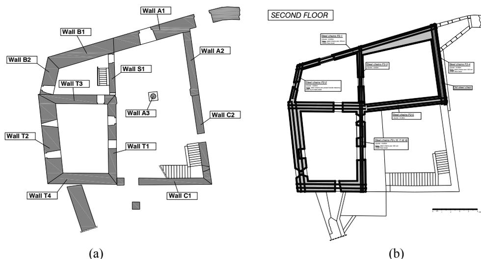
Figure 4 : (a) Elementary walls; (b) Steel chains on second floor
