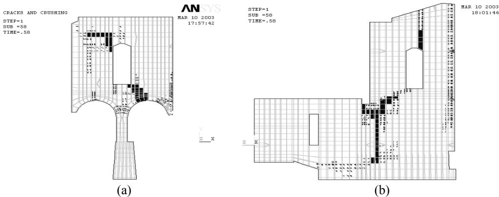
Figure 6 : (a) Cracking path on Wall A3; (b) Cracking path on Wall A2/C2
