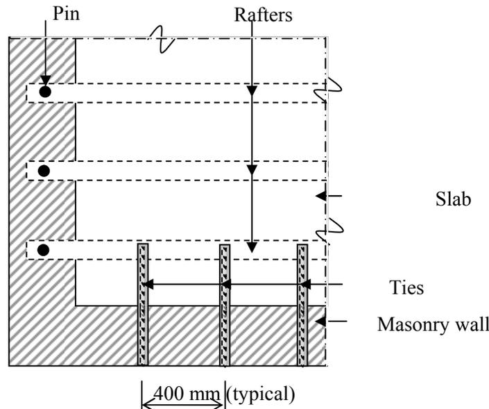
Figure 4 : Typical strengthening of a slab-to-wall connection at a corner.
