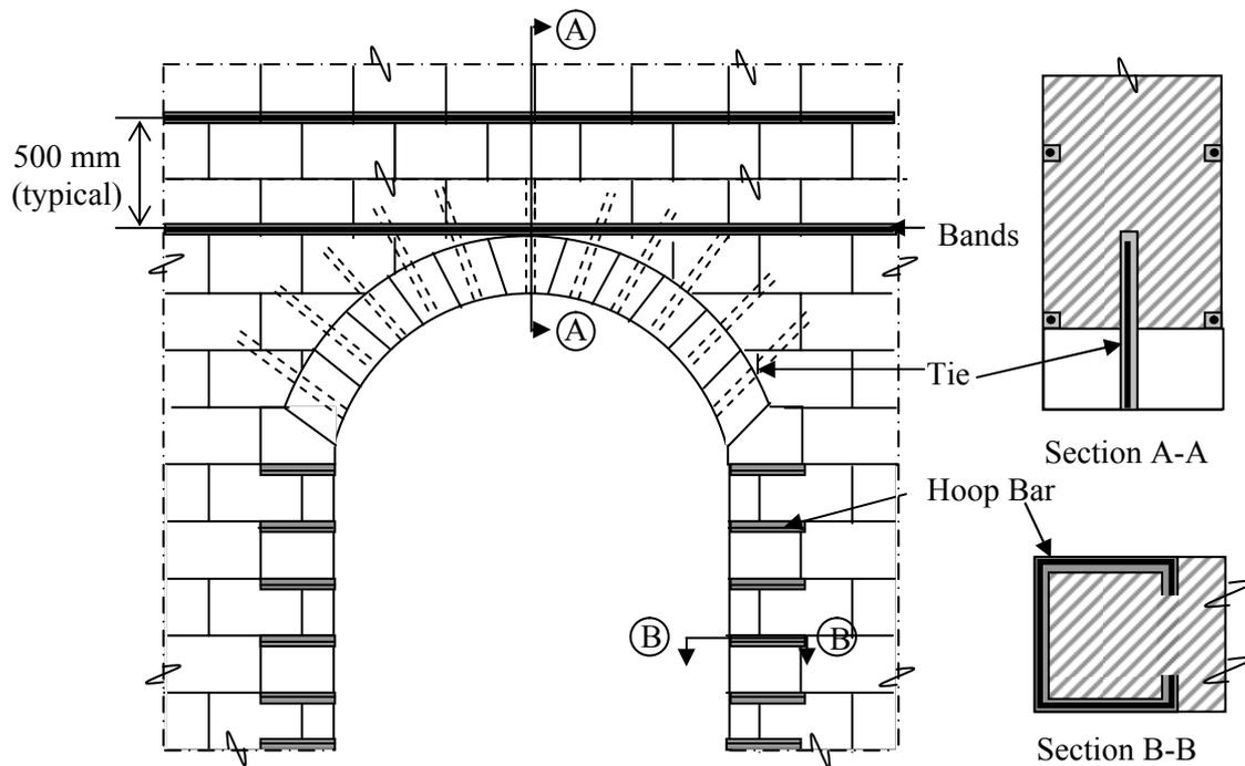
Figure 5 : Typical strengthening of cracked arches.
