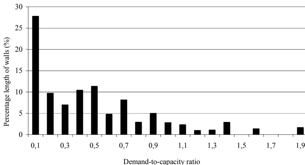
Figure 3 : Percentage length of walls versus demand-to-capacity ratio.
