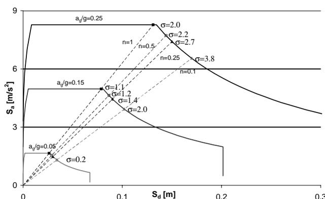
Figure 10 : A.D.S.R. plot of tensile stress evolution ( $\sigma$  in MPa) with aging and several P.G.A. values.
