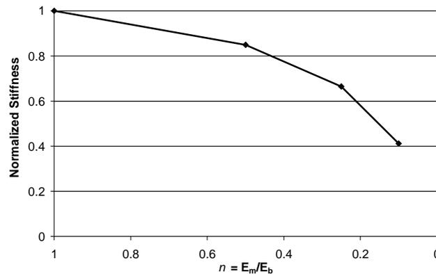
Figure 8 : Normalized stiffness reduction vs.  $n$  ratio (aging).
