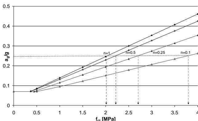
Figure 9 : P.G.A.s vs. minimum tensile strength requirement.
