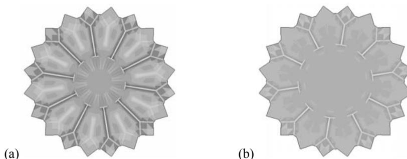
Figure 7 : Vertical stress Contour Plot. Horizontal sect. ( $n=0.25$ ): (a) aligned pattern, (b) Pompeii's pattern.
