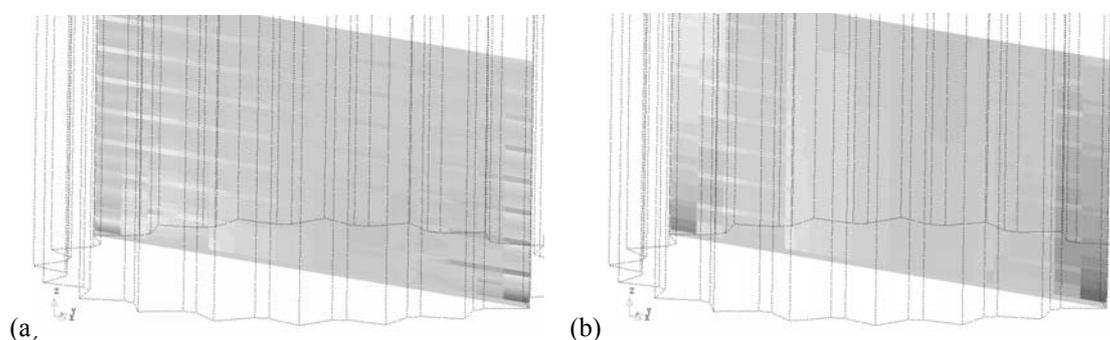
Figure 6 : Vertical stress Contour Plot. Vertical sect. ( $n=0.25$ ): (a) aligned pattern, (b) Pompeii's pattern.
