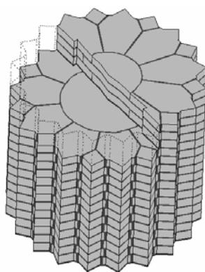
Figure 5 : A segment of the F.E.M. micro-scale model adopted: Pompeii's pattern detail.
