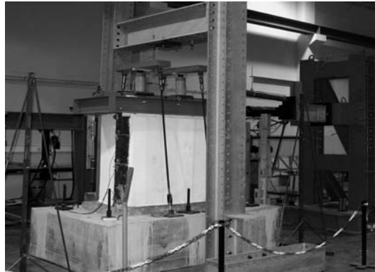
Figure 2 : Wall view and testing scheme.
