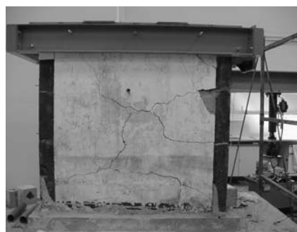
Figure 6: Wall façade after the experiment.
