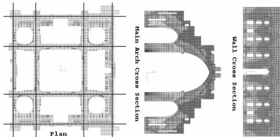
Figure 5 : Lateral load resistant cross sections for Fatih mosque
