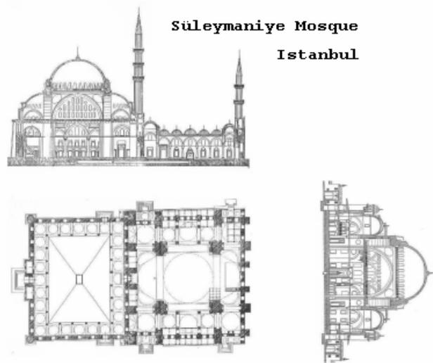
Figure 1: Square Support system for the dome, arches on two sides, semi-domes on two sides.
