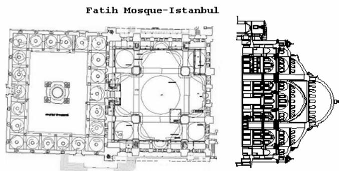
Figure 2 : Square support system for the dome, semi-domes on four sides.
