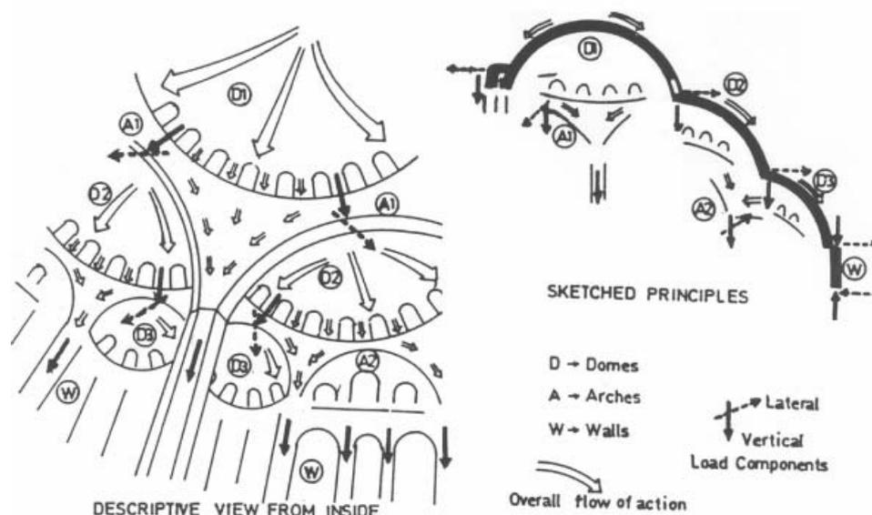
Figure 4 : Gravity load transfer mechanism in Ottoman domes (Karaesmen and Unay 1988 )
