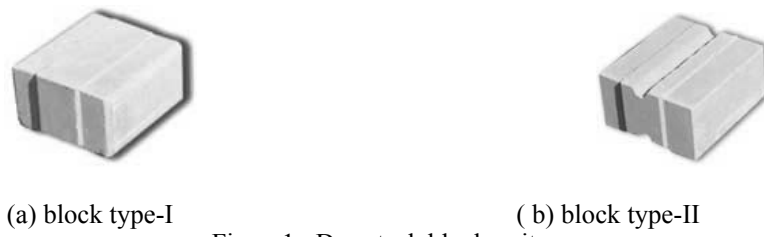
Figure1 : Dry-stack block units
