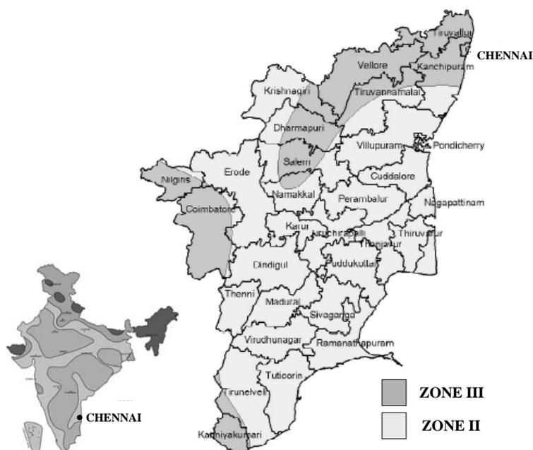
Figure 1 : Seismic hazard zonation for the State of Tamil Nadu (BIS-1893:2002, Source: BMTPC, India)
