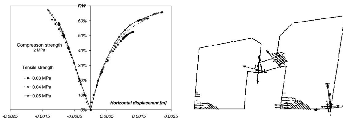
Figure 4 : 2D sensitivity analysis and plastic strains in the wall 1 of “S. Angelo mill” (Ottati).
