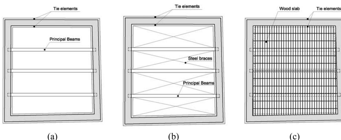
Figure 2 : The different retrofit techniques: (a) connection of the wooden beams to the masonries; (b) bracing reinforcement of the timber slab; (c) insertion of a timber double crossed slab.
