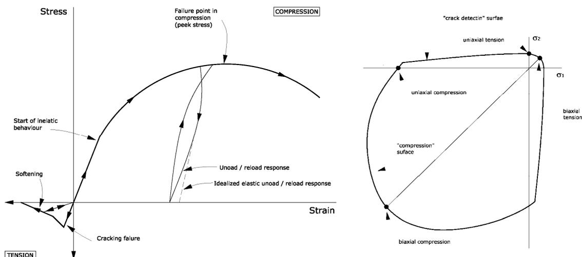
Figure 3 : A stress-strain curve and two-dimensional failure surface for masonry.
