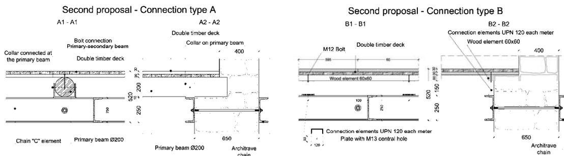
Figure 9 : Second connection solution – One way floor with double timber deck.
