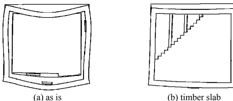
Figure 5 : Comparison between the deformed shape of the “as is” mill and the mill with a timber slab.
