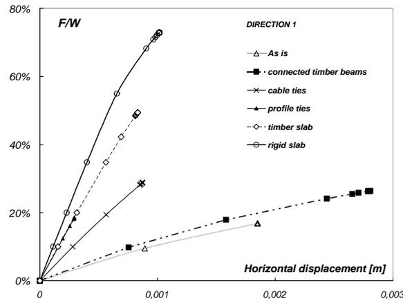
Figure 6 : Collapse multiplier for the different retrofit techniques models of the “Mill B”.
