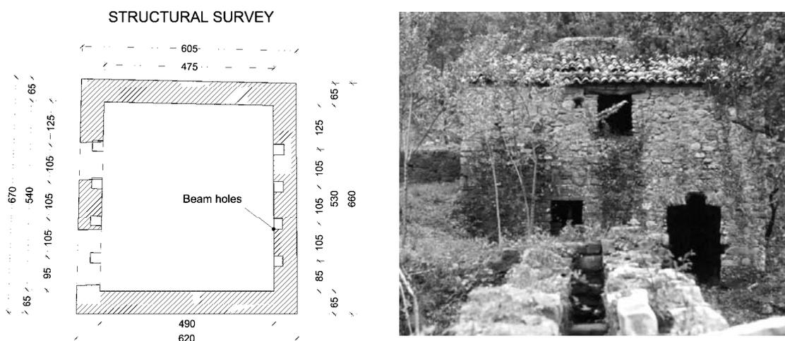
Figure 1 : The mill masonry structure namely “Mill B” located in Perdifumo.
