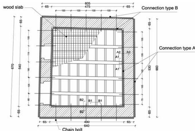
Figure 7 : Slab restoration layout.
