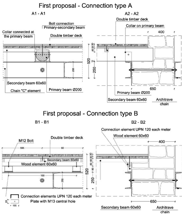
Figure 8 : First connection solution – Two way floor with double timber deck.
