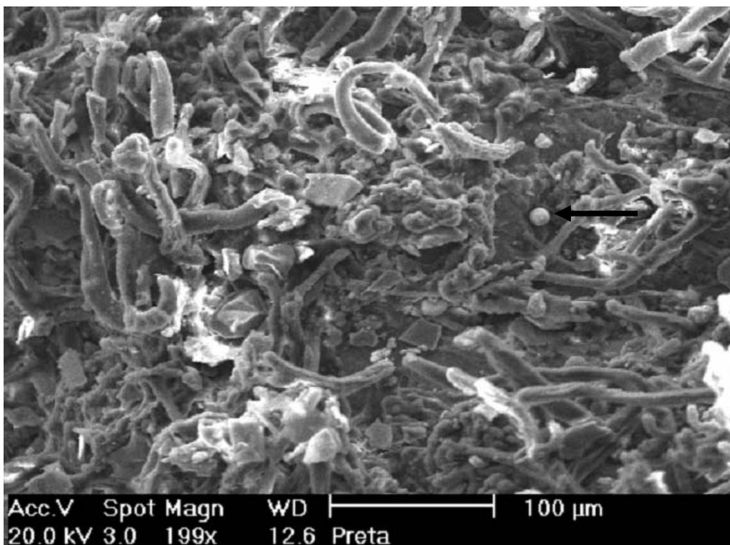
Figure 2 : Scanning electron micrograph of patina on the quartzite parapet of the church. Arrow indicates spherical cells in a similar sized pit.
