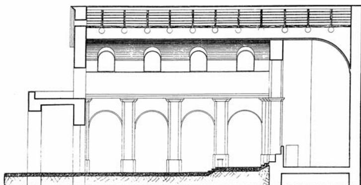
Figure 3 : Longitudinal section of the Church.
