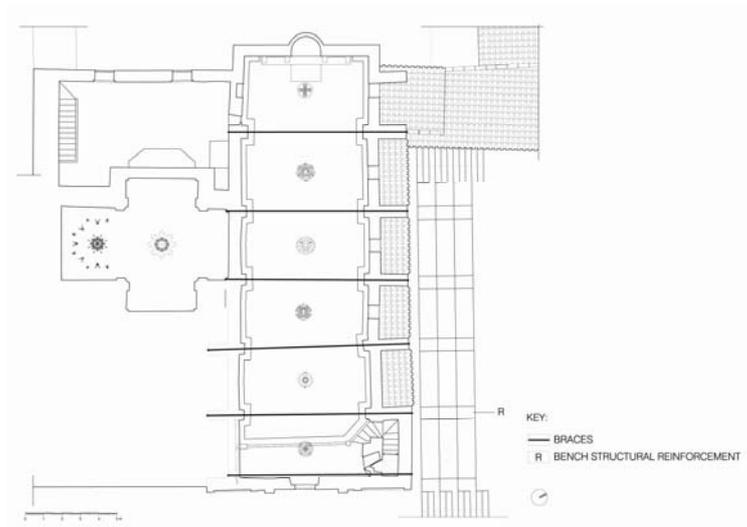
Figure 7 : Solution of braces and reinforcement.
