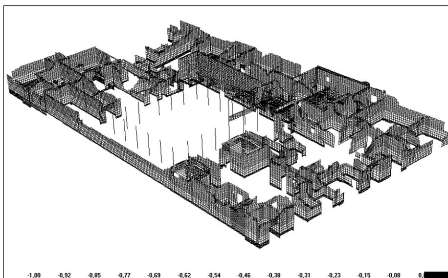
Figure 3 : Response to the seismic load in x-direction in the actual configuration.
