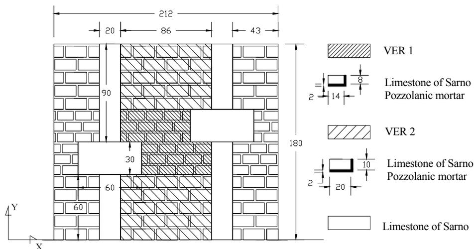
Figure 1 : Volume of reference for the masonry called ‘opera a telaio’.
