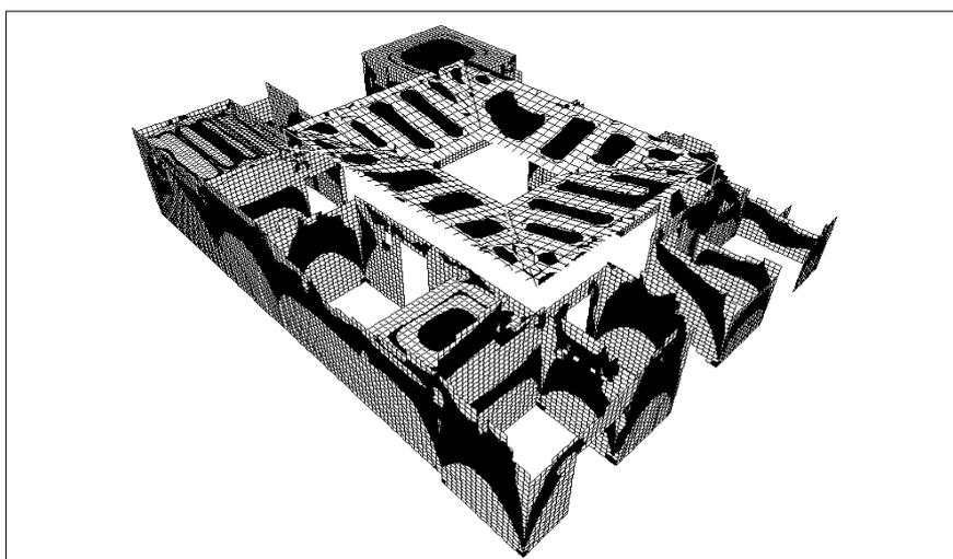
Figure 5 : Model of the main atrium with a new cover : map of the stresses due to wind.
