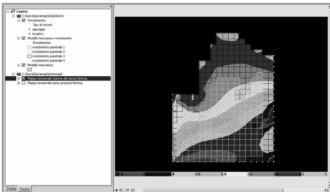
Figure 7 : View of 21c wall with its stress map due to an earthquake.
