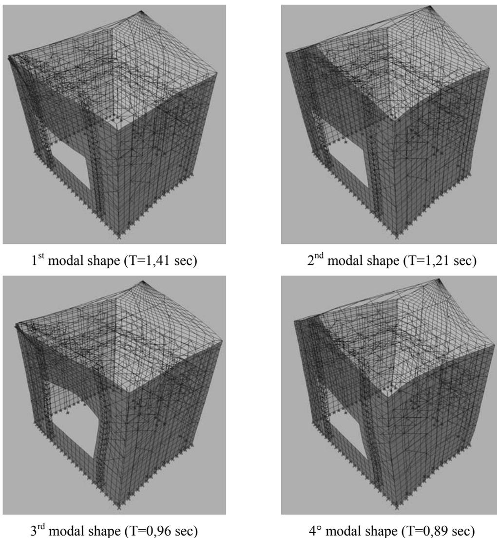
Figure 6 : the first modal shapes of the structure.
