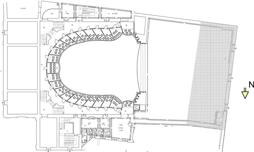
Figure 1 : The floor plan of "Teatro Zandonai": the 18<sup>th</sup> century enlargement is highlighted.
