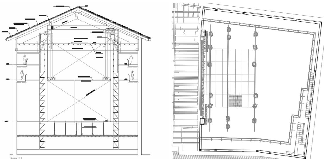
Figure 4 : Floor plan and section of the earthquake resistance steel structure for the fly tower.
