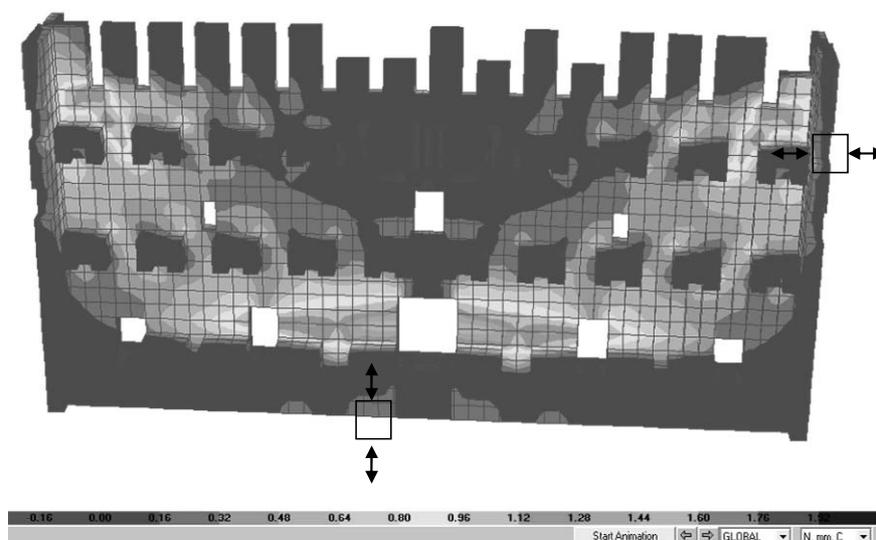
Figure 5 : Maximum (tensile) stresses generating at the stage wall due to sound induced forces
