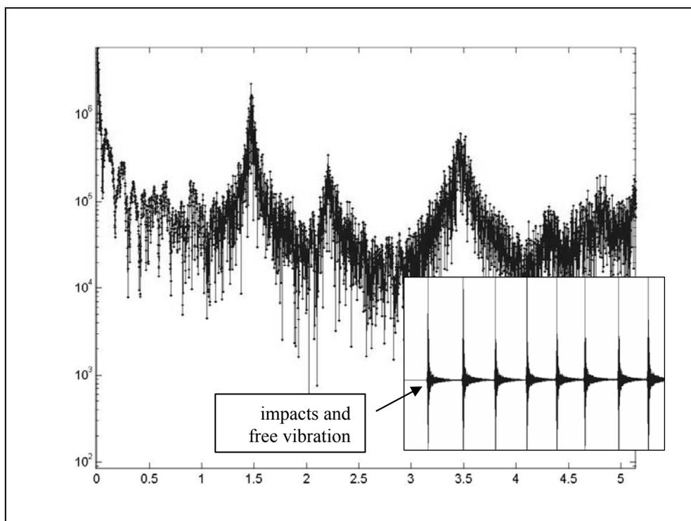
Figure 3 : FFT conversion of recorded impact free vibration data showing resonant frequencies.
