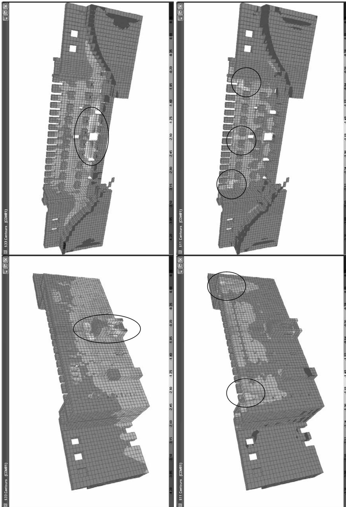
Figure 6 : Maximum (tensile) stresses generating at walls due to DL+EQ induced forces
