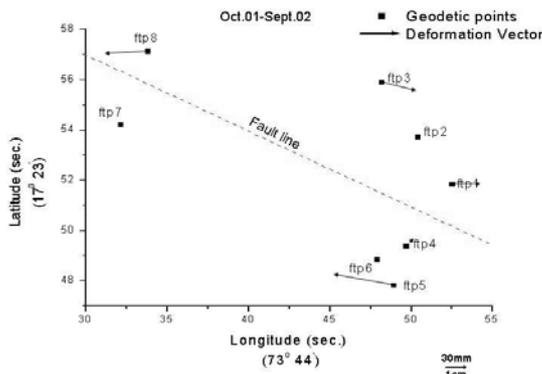
Figure 4 : Deformation vectors of the geodetic points along Koyna Fault from Oct.01 to Sept.02.
