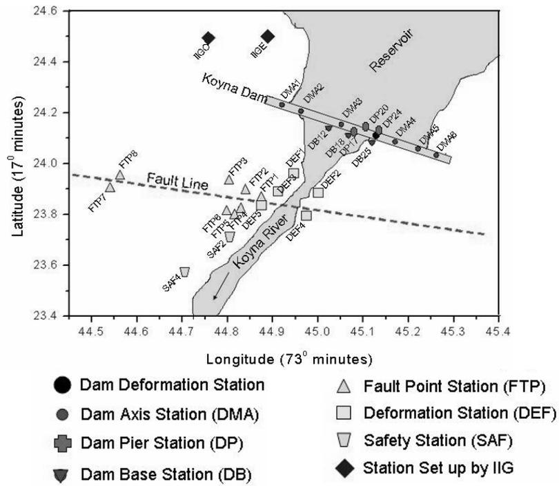
Figure 1 : Distribution of GPS network around the Fault and Koyna Dam area.
