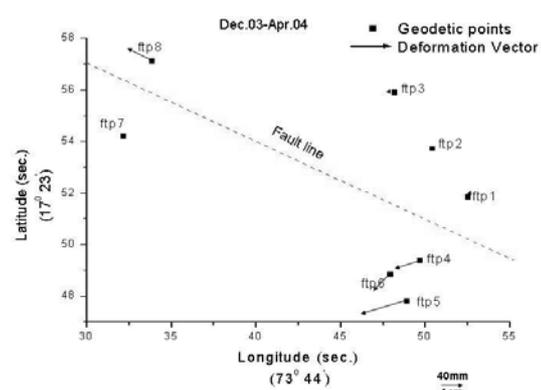
Figure 9 : Deformation vectors of the geodetic points along Koyna Fault from Dec.03 to Apr. 04.
