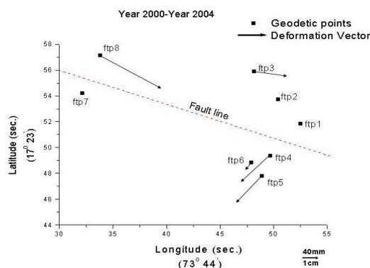
Figure 11: Deformation vectors of the geodetic points along Koyna Fault from Dec.00 to Sept.04.
