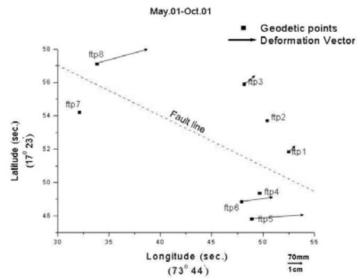
Figure 3 : Deformation vectors of the geodetic points along Koyna Fault from May.01 to Oct.01.
