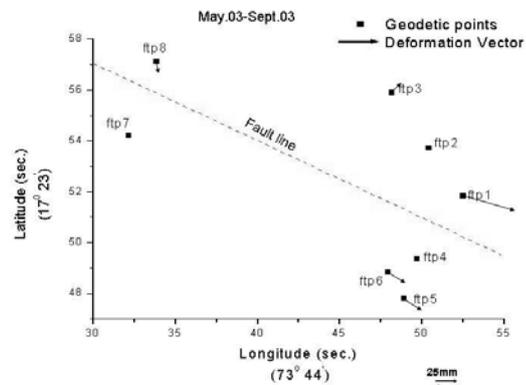
Figure 7 : Deformation vectors of the geodetic points along Koyna Fault from May.03 to Sept.03.
