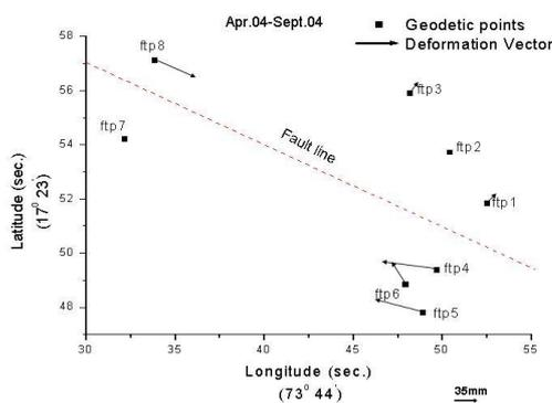
Figure 10 : Deformation vectors of the geodetic points along Koyna Fault from Apr.04 to Sept.04.
