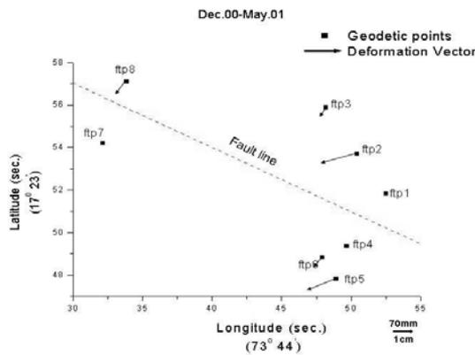
Figure 2 : Deformation vectors of the geodetic points along Koyna Fault from Dec.00 to May.01.
