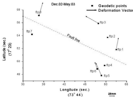
Figure 6 : Deformation vectors of the geodetic points along Koyna Fault from Dec.02.to May.03.
