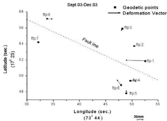
Figure 8 : Deformation vectors of the geodetic points along Koyna Fault from Sept.03 to Dec.03
