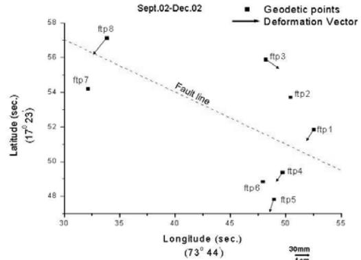
Figure 5 : Deformation vectors of the geodetic points along Koyna Fault from Sept.02 to Dec.02..
