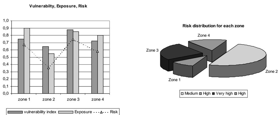
Figure 7 : Indices of vulnerability, exposure and risk for each of the 4 zones (left); percentual distribution of the risk over the wall surface under examination (right).
