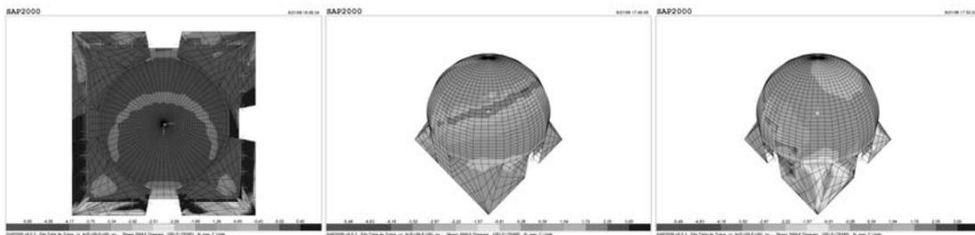
Figure 15 : Bottom and 3D views of resulting SMAX diagrams of the superstructure with concrete cover for the case that the moments of inertia of critical frames were reduced to  $10^8 \text{ mm}^4$  (under dead load and  $25^\circ\text{C}$  randomly distributed temperature load)
