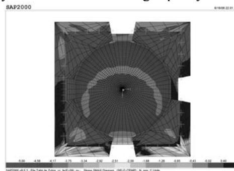
Figure 12 : Bottom view of resulting SMAX diagrams of the superstructure with concrete cover (under dead load and 25°C randomly distributed temperature load)
