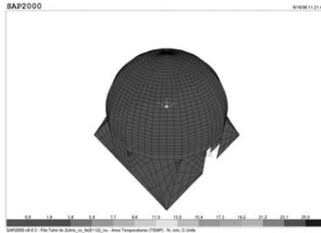
Figure 10 : Applied temperature load of 25°C. Dark blue indicates the part warmer.
