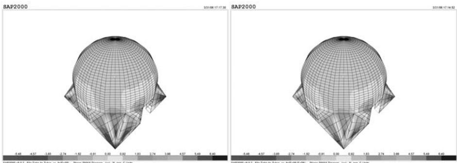
Figure 8 : 3D Smax diagrams for the case that the moment of inertia of the system is  $10^9 \text{ mm}^4$  and that of critical frames were reduced to  $10^8 \text{ mm}^4$  respectively
