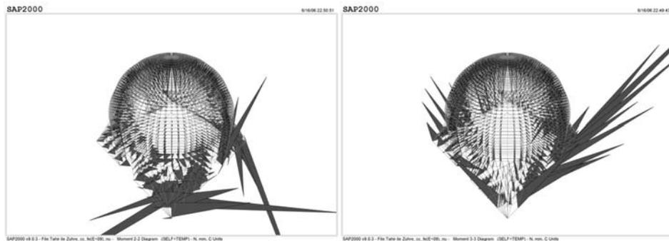
Figure 14 : Resulting 3D moment diagrams in 1-3 and 1-2 directions, respectively (under dead load and  $25^\circ\text{C}$  randomly distributed temperature load;  $I=10^9 \text{ mm}^4$ )
