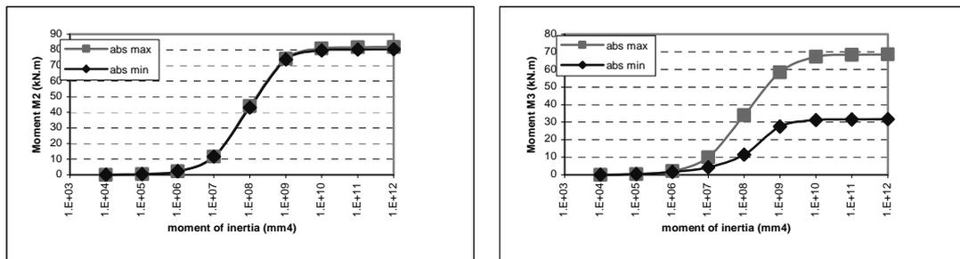
Figure 11 : Graphs of minimum and maximum M2 and M3 values (i.e. bending moments in the 1-3 and 1-2 planes with square and diamond markers, respectively) as a function of moment of inertia.
