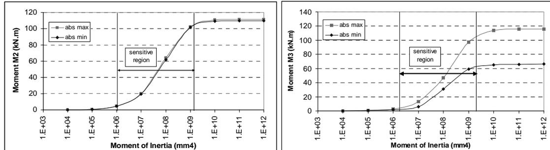
Figure 5 : Graphs of minimum and maximum M2 and M3 values (i.e. bending moments in the 1-3 and 1-2 planes with square and diamond markers, respectively) as a function of moment of inertia (under dead load and 40°C uniform temperature load)
