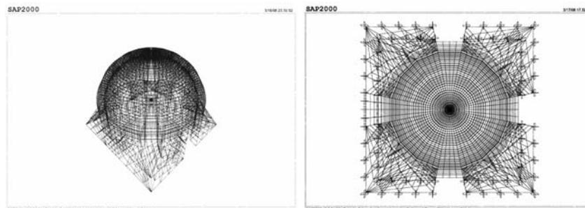
Figure 4 : A 3D view and bottom view of the superstructure composed of two layers connected with rigid links to analyse under temperature load
