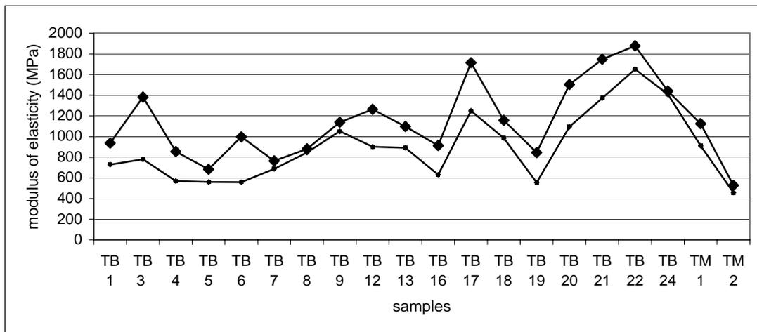
Figure 2 : Variation in modulus of elasticity (Young's Modulus) values (MPa) of the samples in dry and wet state (dry and wet states are shown with diamond and square marks, respectively)
