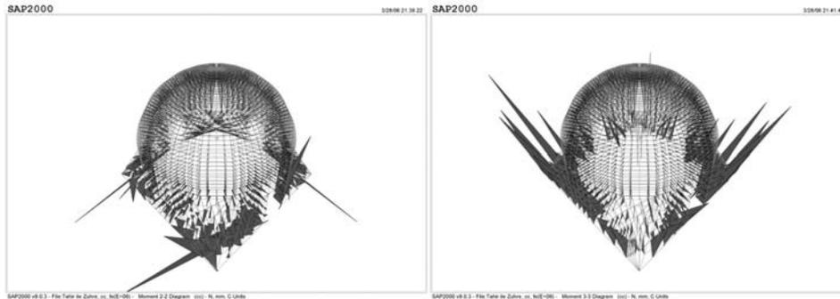
Figure 7 : Resulting 3D moment diagrams in 1-3 and 1-2 directions, respectively (under dead load and 40°C uniform temperature load;  $I=10^9 \text{ mm}^4$ )
