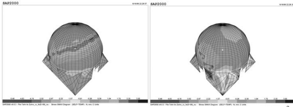
Figure 13 : 3D Smax diagrams for the case that the moment of inertia of the system is  $10^9 \text{ mm}^4$
