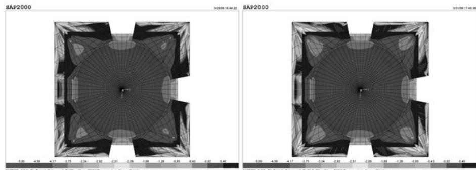
Figure 9 : Bottom views of Smax diagrams when moment of inertia ( $I$ ) is  $10^9 \text{ mm}^4$  and  $I$  of critical frames reduced to  $10^8 \text{ mm}^4$ , respectively
