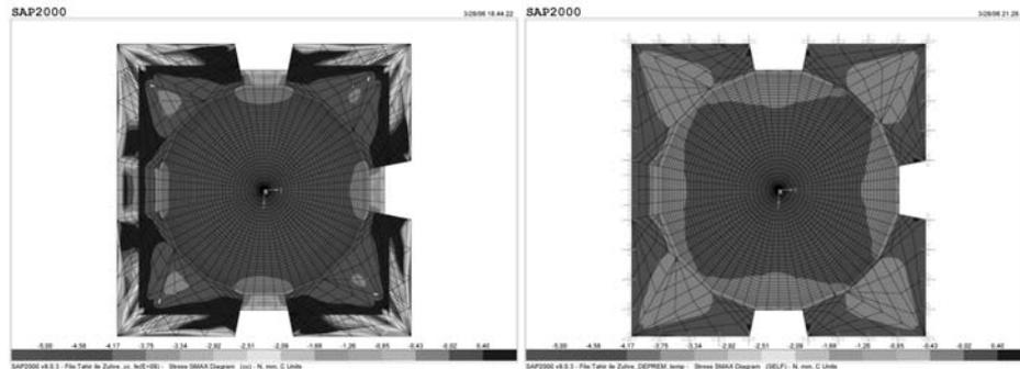
Figure 6 : Bottom view of resulting SMAX diagrams of the superstructure with and without concrete cover, respectively (under dead load and 40°C uniform temperature load;  $I=10^9 \text{ mm}^4$ )
