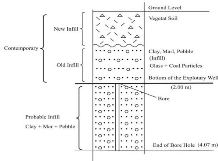
Figure 4 : Section through the exploratory well no 2.
