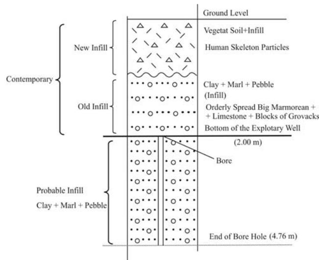
Figure 3 : Section through the exploratory well no 1.
