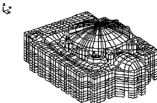
Figure 7 : Finite element modeling of the building.
