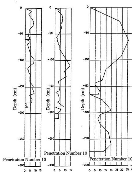
Figure 5 : Penetration values obtained from the exploratory wells.
