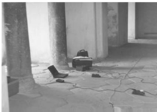
Figure 6 : Free vibration measurements of the Church of St. Sergius and Bacchus (Readings at the gallery floor).
