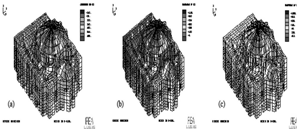
(Static Analysis-Dead Load Only-kN/m<sup>2</sup>-Slice in X-Dir.)
