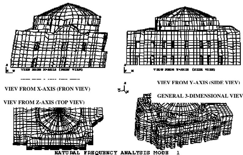
Figure 8 : First mode of the structure.
