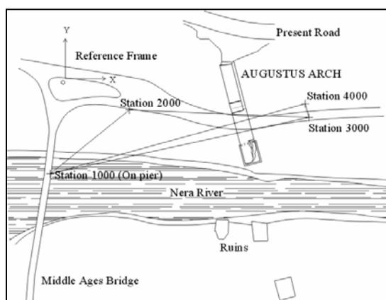
Figure 2 : Top view of the four fixed stations mesh, used in the survey of the Augustus Bridge
