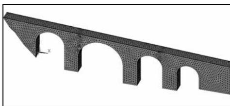
Figure 6 : The 3D model of the Augustus Bridge mesh
