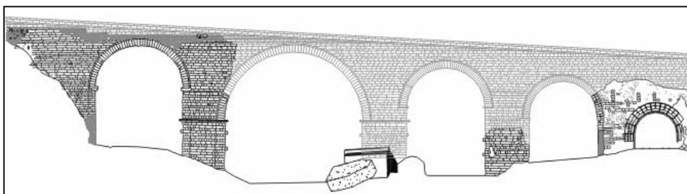
Figure 5 : The front of the virtually reconstructed Augustus Bridge. In black the survey
