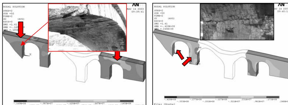
Figure 8 : The strain graph of the remains of the Augustus Bridge. With arrows there have been evidenced the more strained areas.
