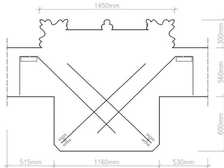
Figure 3 : Cross section of the pillar with reinforcement
