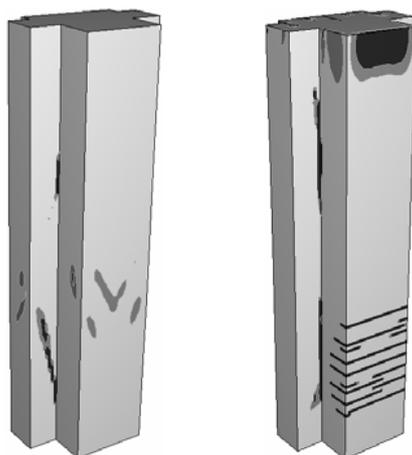
Figure 8 : Pillar failure scheme: (a) perfect geometry, (b) real deformed structure
