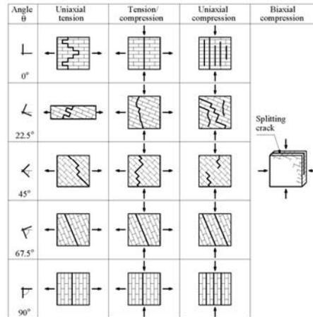
Figure 6 : Typical failure models in terms of principal stresses (Lourenço 1996)
