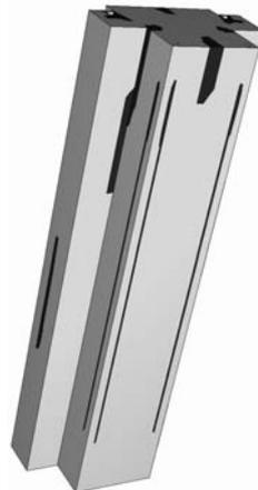
Figure 10: Crack pattern in of reinforced model
