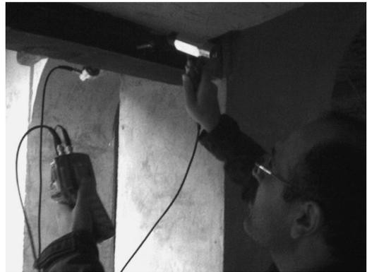
Figure 3. Measuring the transmission time of stress waves.
