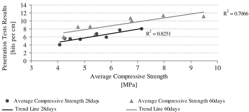
Figure 3. Trend lines. Average Compressive Strength – Penetration tests results (28 days and 60 days).
