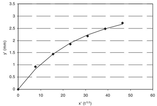
Figure 9. Fitting of data to an exponential curve; data of mortar with binder 1, vacuum pressure 200 mbar.
