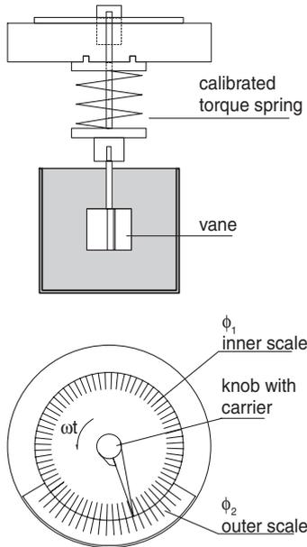
Figure 2. Working principles of the soil vane test.
