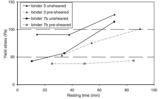
Figure 5. Yield stress unsheared and pre-sheared for air entrained mortars.
