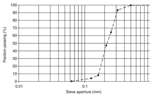
Figure 1. Grading of the aggregate (Zutendaal sand).
