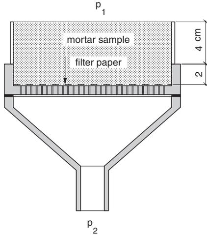
Figure 4. Geometry of the descriptivity test. The section of the dish is circular, diameter 155 mm.
