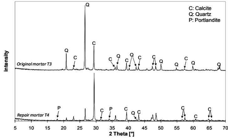
Figure 3: XRD patterns of original mortar T3 (top) and repair mortar T4 (bottom).
