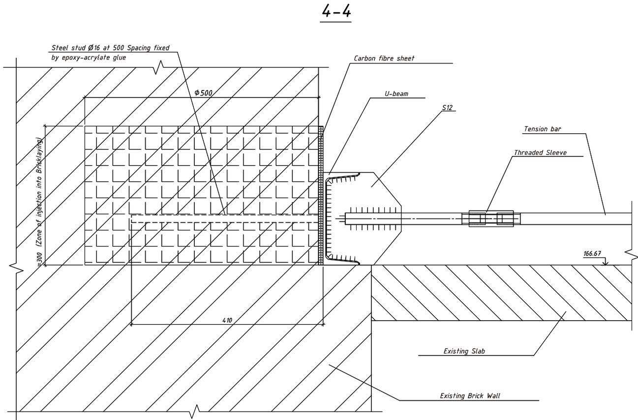
*Figure 3: Attachment between a load-distributing beam and a structural wall*
