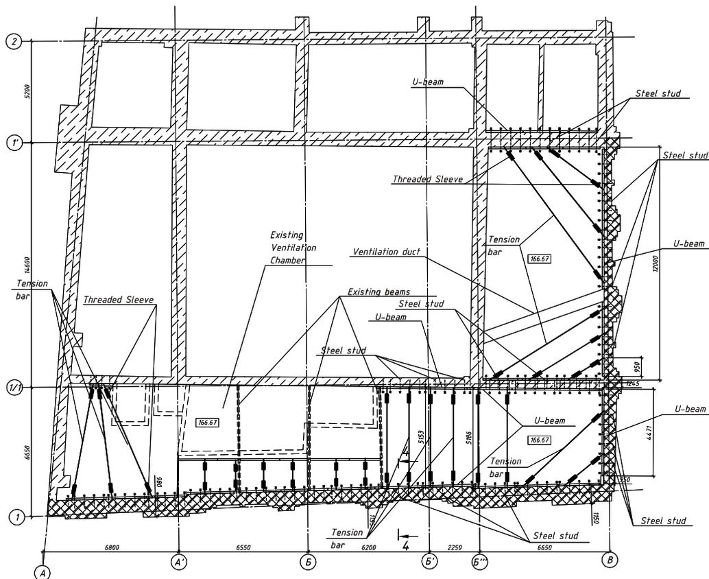
Figure 2: Section of a plan view of the building
