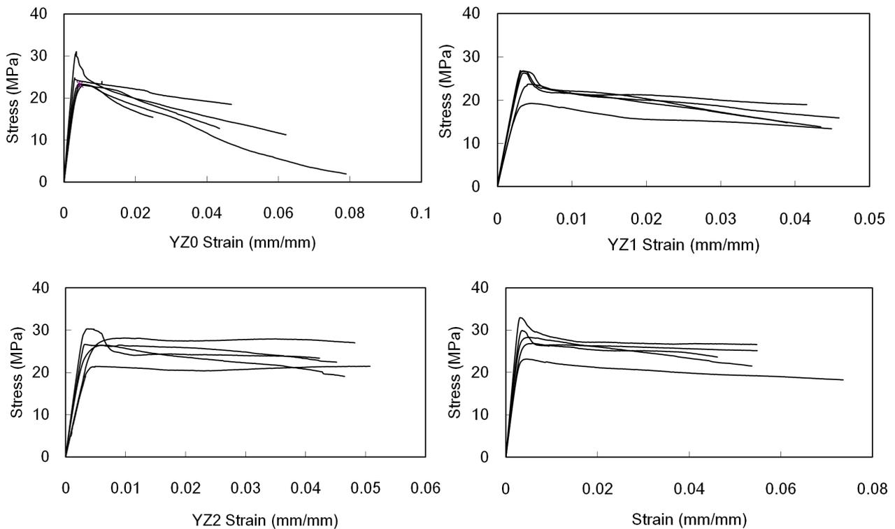
*Figure 6: Longitudinal stress and strain relationship of wood cylinders*
