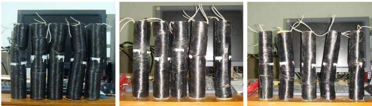
*Figure 5: Failure modes of wood cylinders wrapped with fiber composite sheets*
