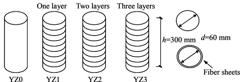
Figure 2: Geometry of the specimens
