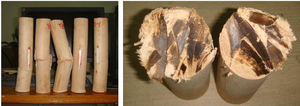
*Figure 4: Failure modes and cut image of wood cylinders without fiber sheets wrapping*
