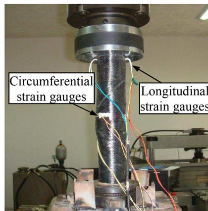
Figure 3: Test setup and strain gauge allocation
