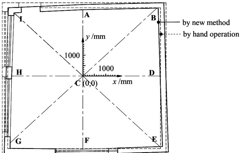
Figure 10: Plans drawn with the new method and the hand operation
