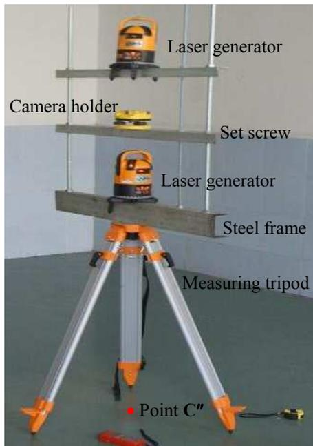
Figure 4: Equipments of the new method
