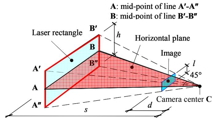
Figure 7: Determination of the distance
