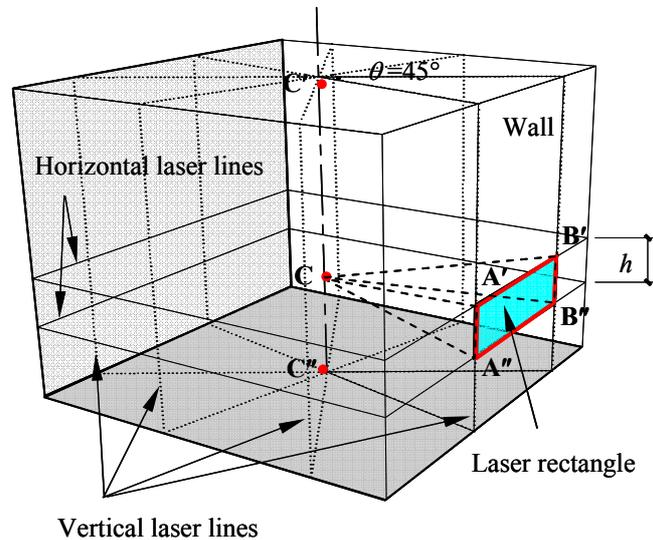
Figure 5: Laser lines on the inner walls
