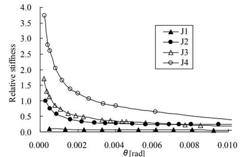
Figure 6: Skeleton curves of load-displacement relationship Figure 7: Stiffness degradation curves
