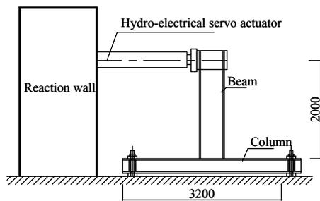
Figure 2: Test setup
