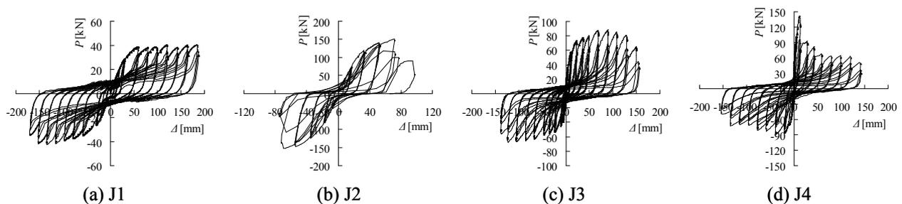
Figure 5: Load-displacement relationships of the specimens
