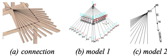
*Figure 5: Analytical model of the Sunjayeon*
