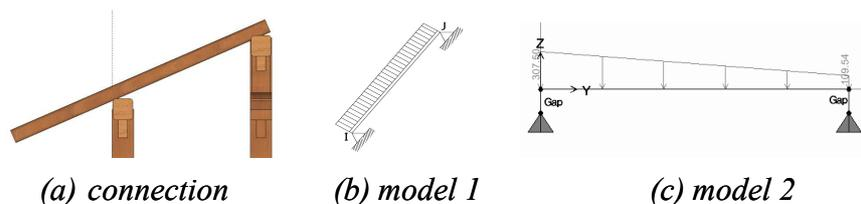
Figure 4: Analytical model of the Danyeon
