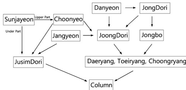
Figure 3: Delivery system of vertical load in the Mindori-House
