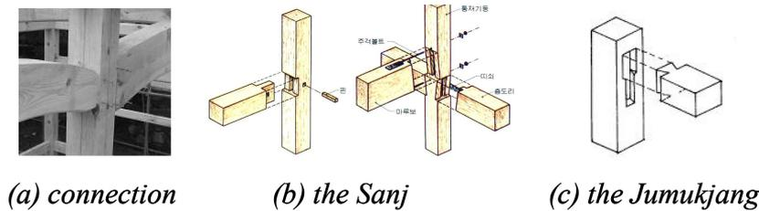
Figure 8: Connecting methods used in the Goju
