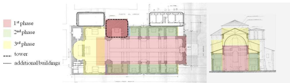
Figure 1: Schematic view (both on plan and section) of the subsequent transformations occurred
