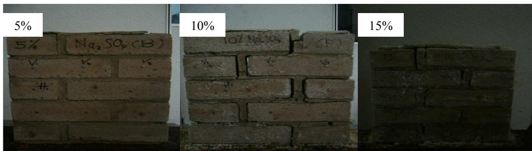
Figure 7: Calcium silicate brickwork after exposed to severe sulphate condition
