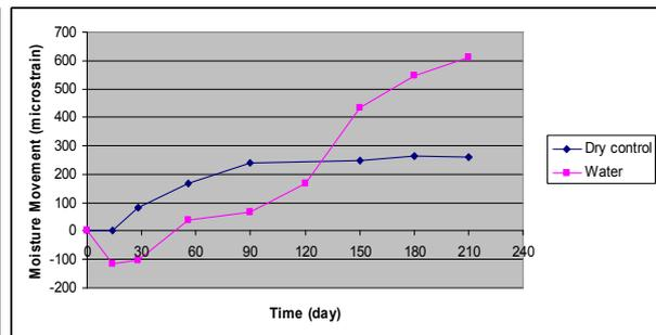
Figure 4: Moisture movement of calcium silicate masonry wall under control condition
