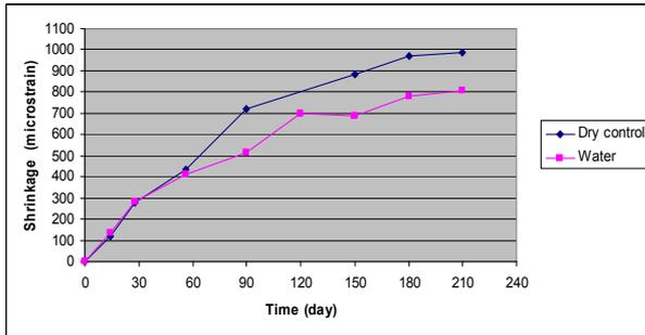
Figure 1: Shrinkage of mortar under control condition
