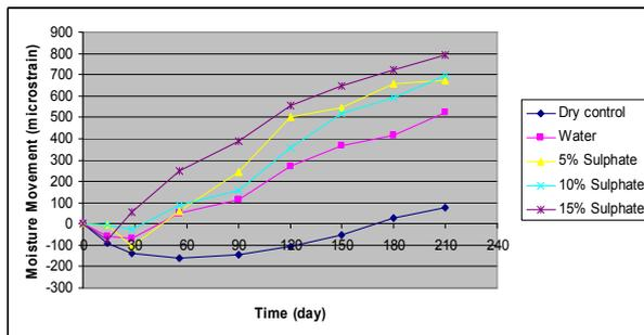
Figure 3: Moisture movement of calcium silicate brick unit
