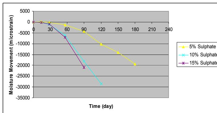
Figure 5: Moisture expansion of calcium silicate masonry wall under sodium sulphate condition
