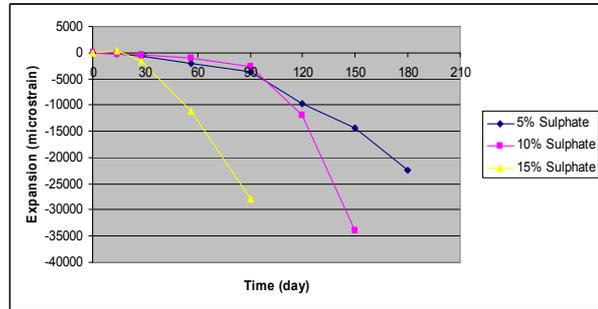
Figure 2: Expansion of mortar prism under sodium sulphate condition
