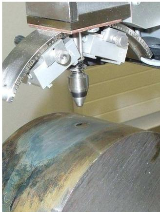
Figure 3: Residual stresses measurements on a steel wheel
