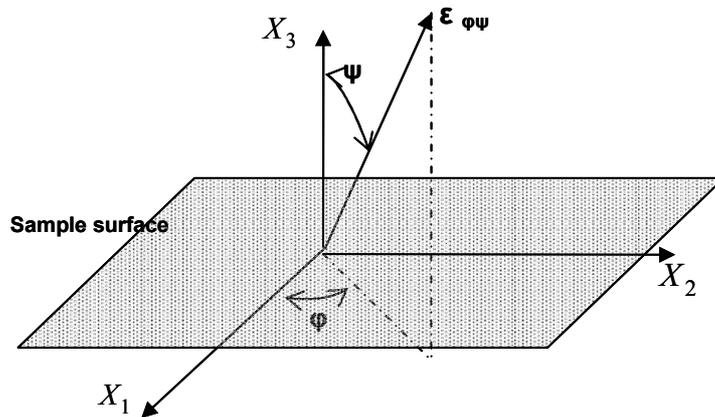
Figure 4:  $\{X_i\}$  represents the reference system fixed over the sample whereas the direction of  $\epsilon_{\phi\psi}$  is coincident with the normal to the diffracting planes
