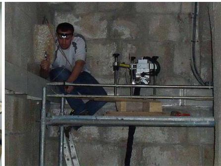
*Figure 6: Load application at the bars in Oporto Cathedral*
