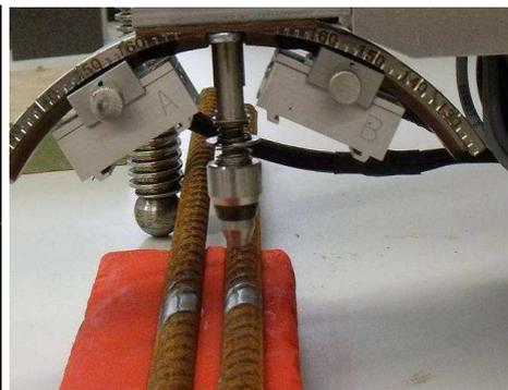
*Figure 8: Sight of the calibration process before loading corrugate bars*
