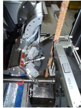
Figure 10: Measurement process on the corrugate bar in tensile machine
