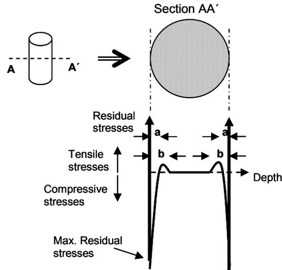
Figure 1: Conventional profile of the residual stresses inside steel bars
