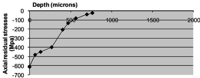
Figure 2: Conventional residual stresses profile in depth
