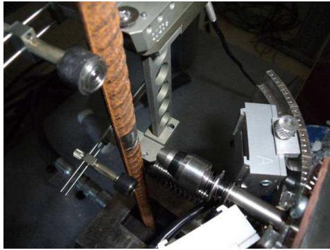
Figure 9: Measurement process on the corrugate bar in tensile machine
