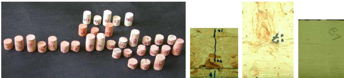
*Figure 3: Set of micro-core specimens and unwrapped surfaces of micro-cores No 22, 37, 61 from layers 5, 6 and 14 respectively*
