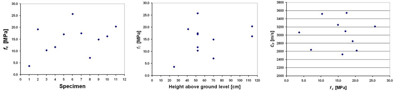
Figure 5: Compressive strength  $f_c$  of brick micro-cores from the Monastery in Supraśl: left – sequence of measured values; center – depending on the height position in the wall; right – compared with velocity of ultrasonic pressure wave  $C_p$
