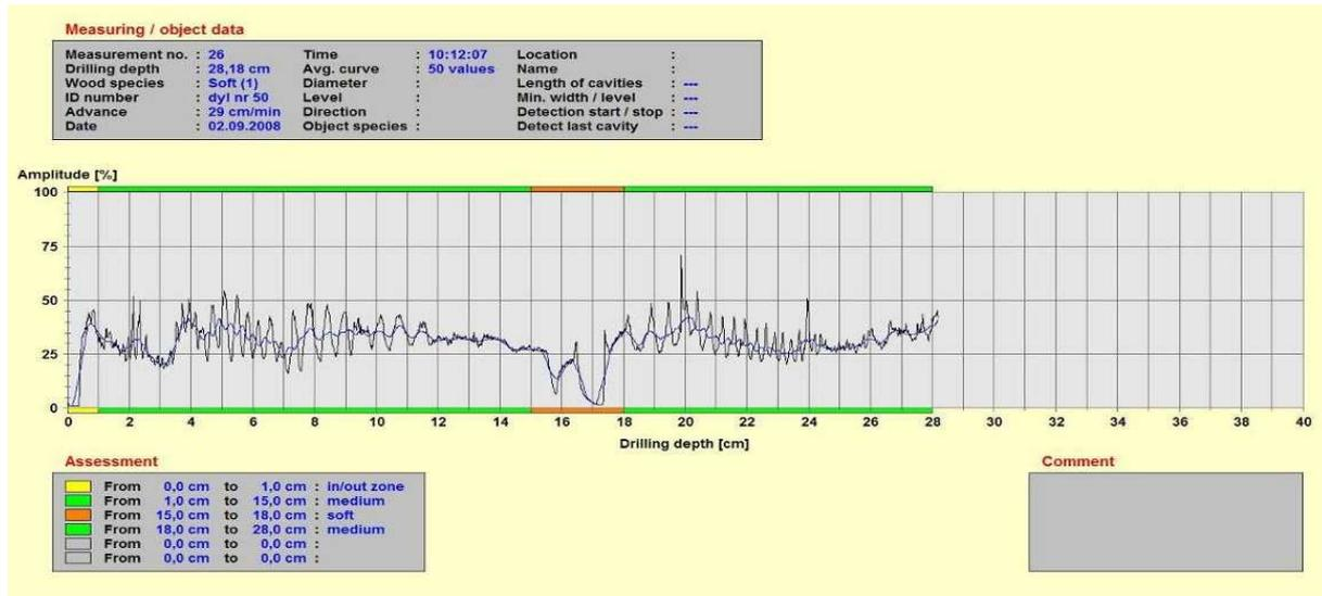
Figure 4: Exemplary resistographic measurement result for ceiling deal (timber beam) above Leopoldinum Auditorium
