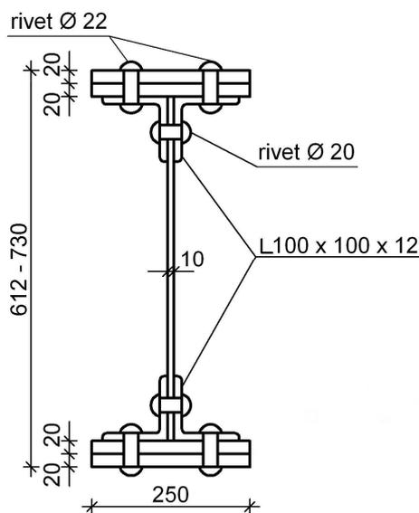
Figure 2: Cross-section of plate girder in span section
