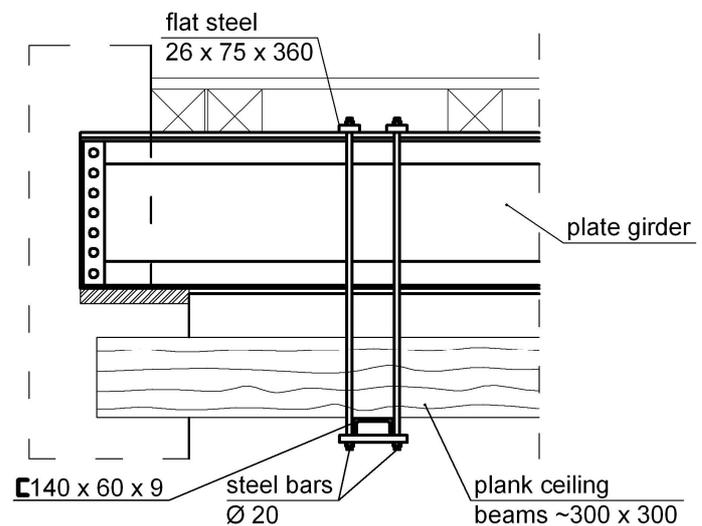
Figure 3: Suspension of deal ceiling from plate girder
