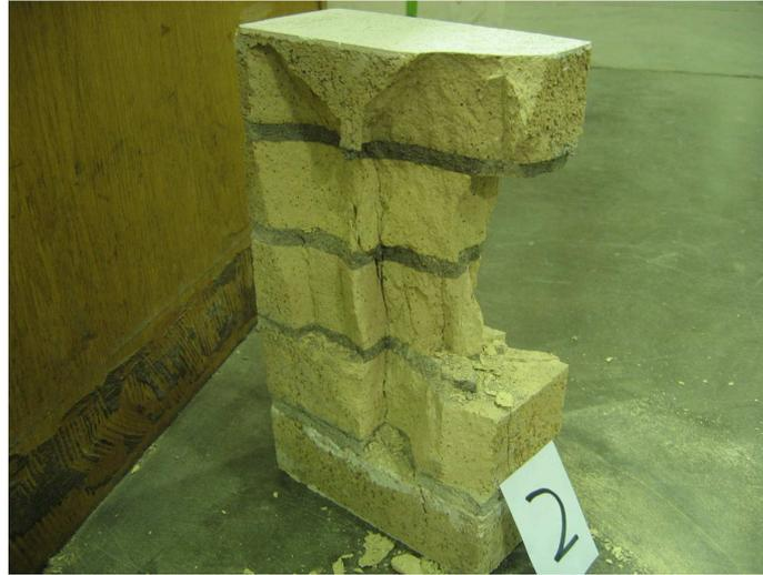
Figure 1: Failure of masonry prism as result of compression test
