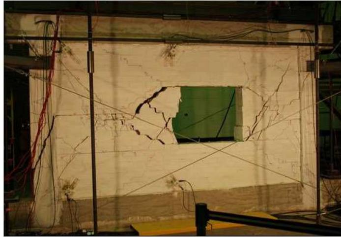
Figure 3: Final crack pattern of infilled frame with eccentric window opening (Blackard et al. 2009)
