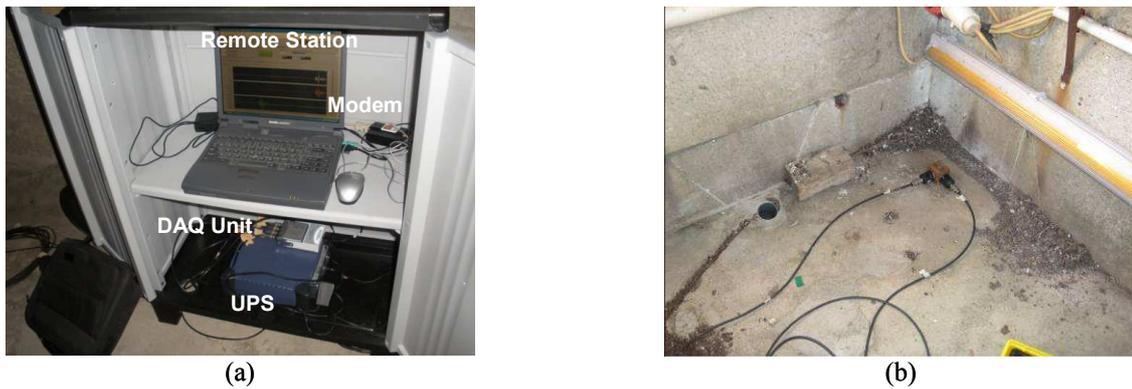
Figure 6: Continuous Dynamic monitoring system setup. (a) Data acquisition station; and (b) measurement node
