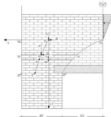
Figure 2: Masonry element with thrust
