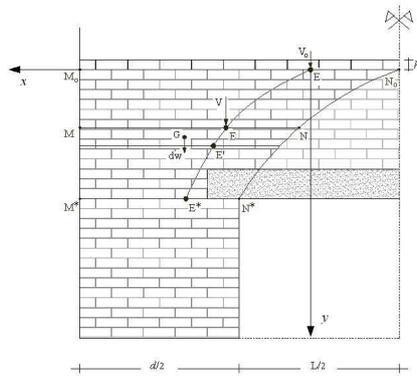
Figure 1: Masonry element without thrust
