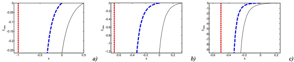
Figure 3: (a)  $d=2L$ ; (b)  $d=L$ ; (c)  $d=0.5L$  (--Lateral profile, - -thrust line, — intrados line)
