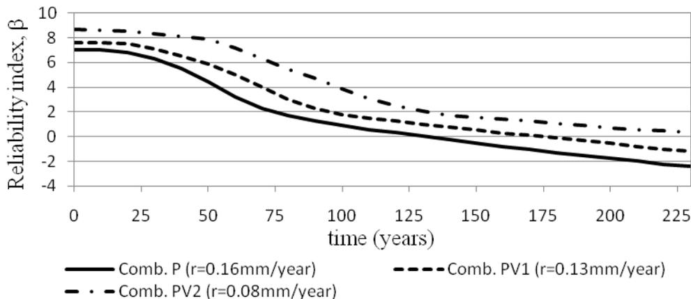
Figure 3: Time evolution deterioration curves for truss 2 and deterministic cross-section model with inspected values
