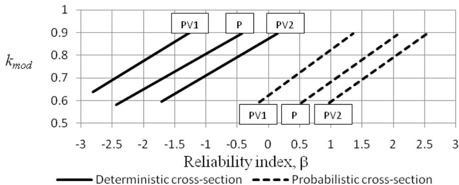
Figure 2: Linear variation of  $k_{mod}$  factor: truss 2
