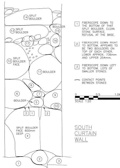
Figure 4: Results of fiberscope probe of South curtain wall (Heritage Conservation Program 2000)
