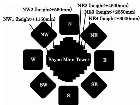
Figure 2: Location of Crack
