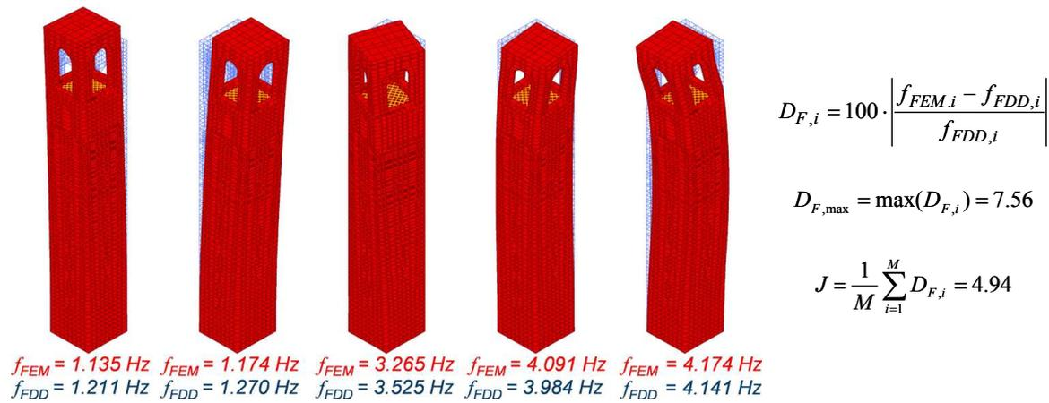
Figure 5: FEM4: vibration modes and comparison with the experimental results
