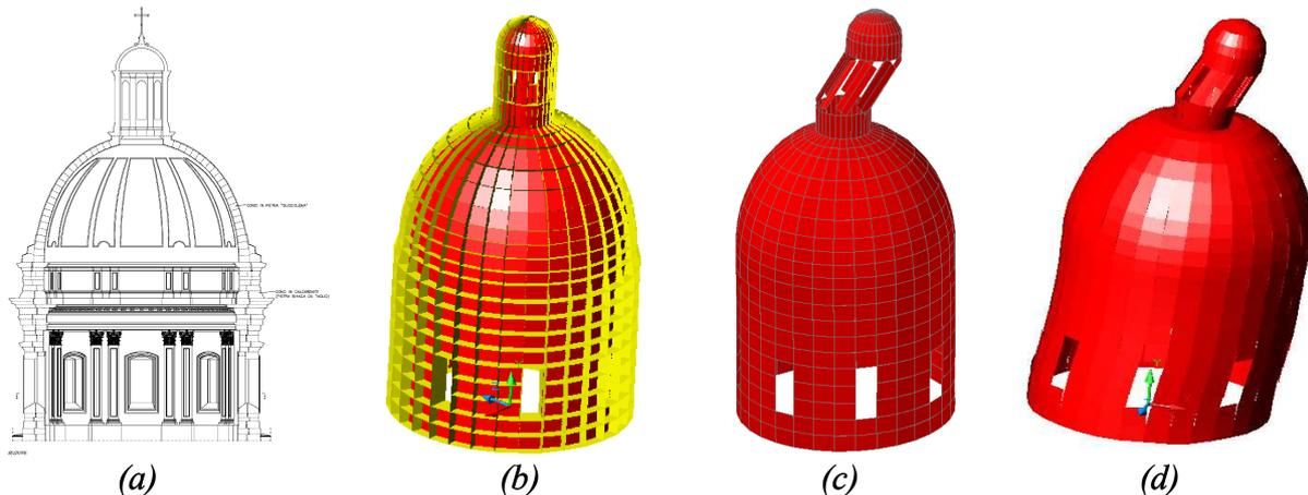
*Figure 6: (a) Section of the dome (figure from reference [9]); (b) The macro-element discretization; (c) the deformed configuration in the condition of incipient collapse considering an unreinforced masonry lantern; (d) the deformed configuration in the condition of incipient collapse considering a linear elastic behaviour of the lantern*
