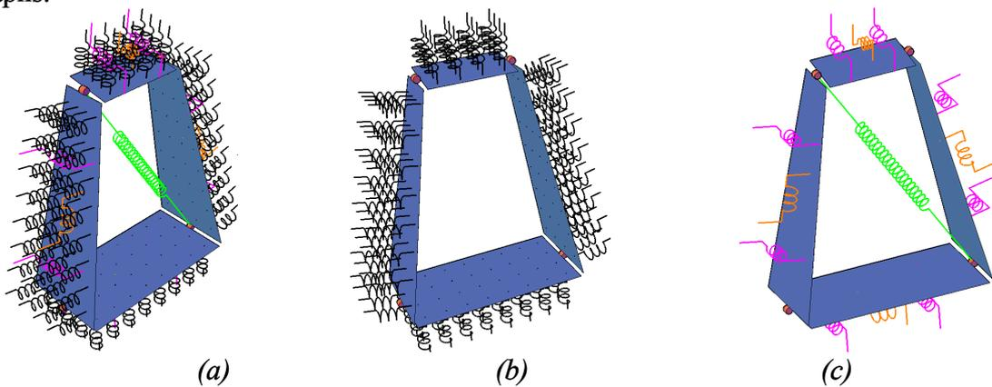
Figure 3: (a) the quadrilateral macro-element 'quad'. (b) the quad with the representation of the orthogonal NLinks for the simulation of membrane and flexural behaviour; (c) the quad with the representation of the transversal and diagonal NLinks for the simulation of shear and torsional behaviour
