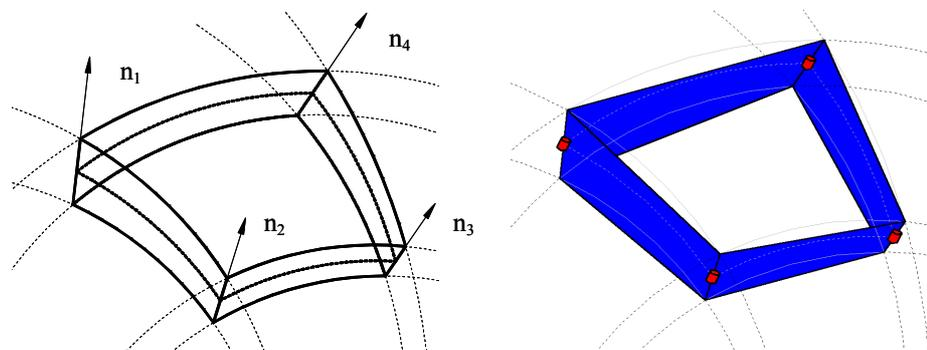
Figure 4: Masonry portion and its equivalent mechanical model without the NLink representations
