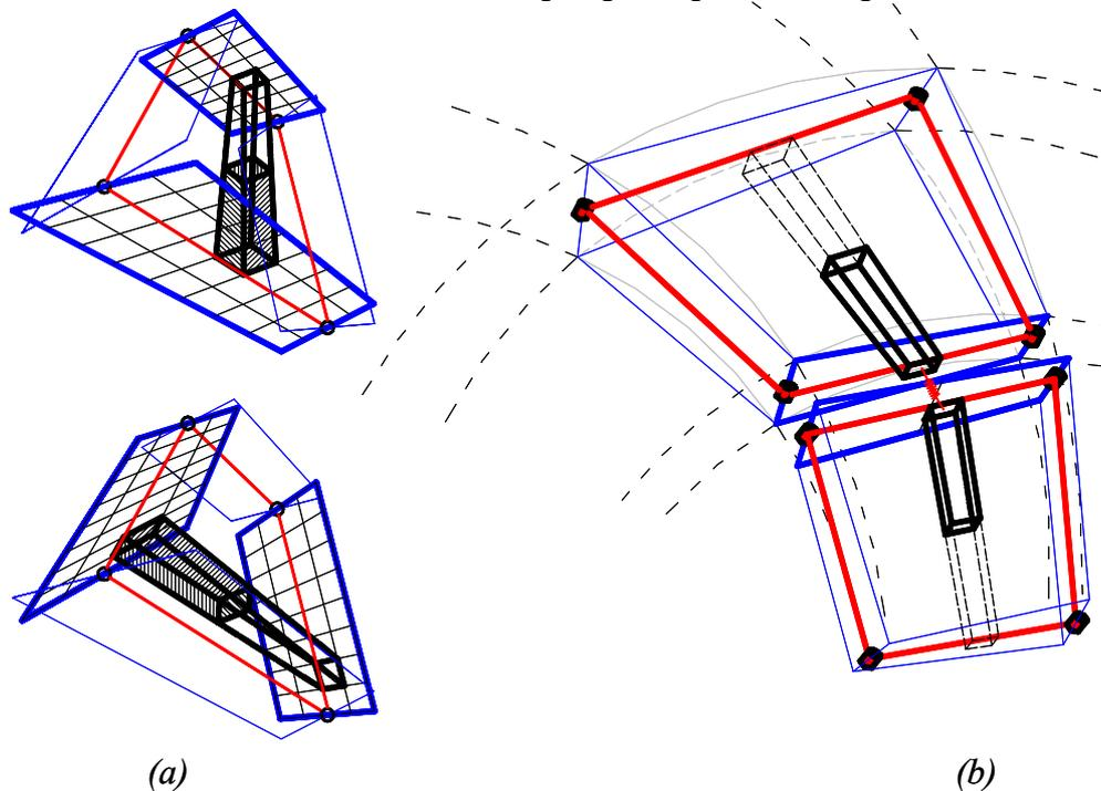
Figure 5: (a) fiber semi-volumes and corresponding nonlinear springs. (b) NLink as a results of two nonlinear springs in series of two adjacent elements
