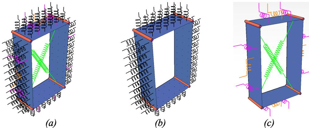
Figure 1: (a) the rectangular macro-element 'rect'. (b) the rect with the representation of the orthogonal NLinks for the simulation flexural behaviour; (c) the rect with the representation of the transversal and diagonal NLinks for the simulation of shear and torsional behaviour
