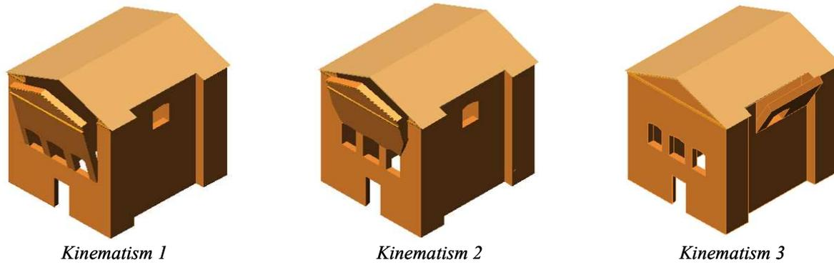
Figure 4: Collapse mechanisms analyzed for the seismic behaviour study
