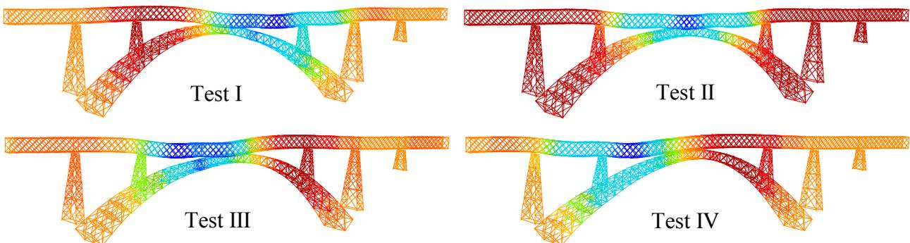
Figure 4: FEM deformed configurations of the try-out tests in Fig. 3 (amplification factor = 250)
