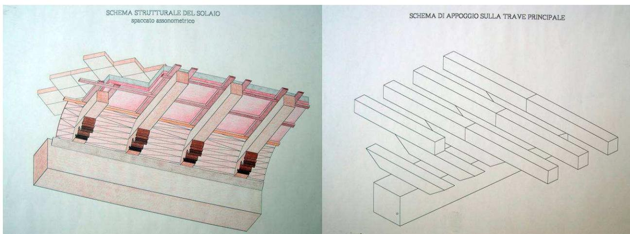
Figure 2: The details of the wooden floor of the main hall
