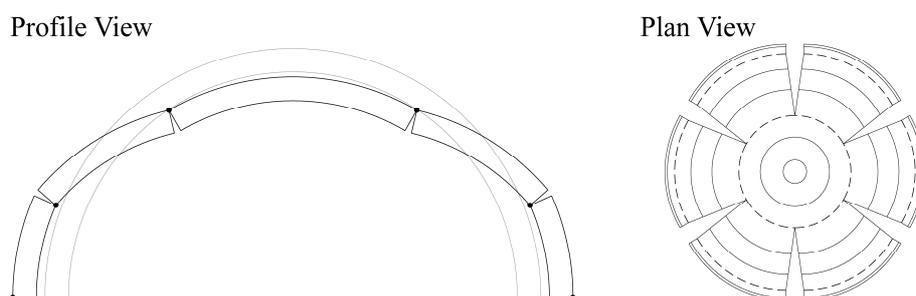
*Figure 4: Symmetrical six-hinge collapse mechanism of dome on spreading supports*
