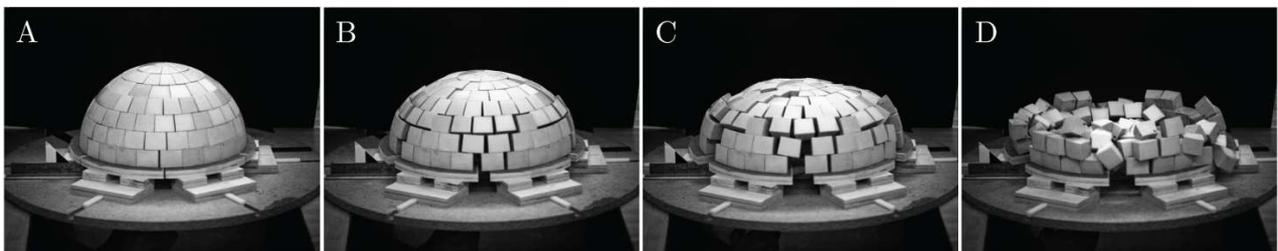
*Figure 3: Still images taken during collapse of Dome 2 with high-speed video*
